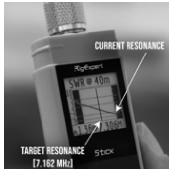
FIG. 2 - Since the target resonance is lower than the current resonance, the tuning collar must be moved down.
