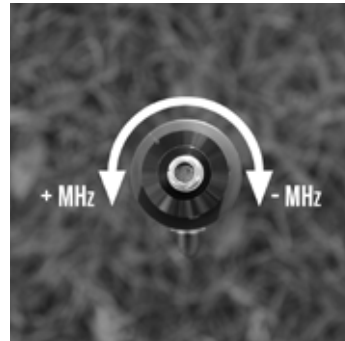
FIG. 3 - Spinning the tuning collar clockwise lowers the resonant point. Spinning the tuning collar counterclockwise increases the resonant point.
