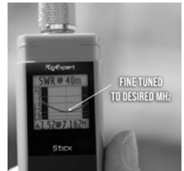
FIG. 4 - After turning the tuning collar the appropriate direction, the resonant point directly aligns with the desired frequency.
