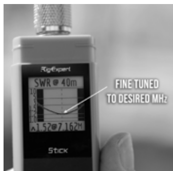
FIG. 4 - After extending/ retracting the whip, the resonant point directly aligns with the desired frequency.
