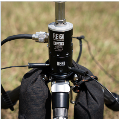
Radials remain connected during antenna changes.
