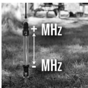
FIG. 1 - Lowering the tuning collar results in a lower MHz resonant point, raising it increases the MHz.
