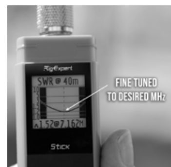
FIG. 4 - After turning the tuning collar the appropriate direction, the resonant point directly aligns with the desired frequency.
